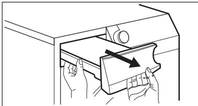
2. Pull the plastic connection out and drain the water into a basin or equivalent receptacle.
