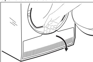
3. Turn the levers to unlock the condenser lid.
