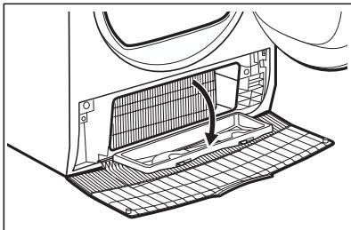
5. If necessary, remove the fluff from the condenser and its compartment. You can use a vacuum cleaner with a brush attachment.
