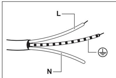
1. Connect the green and yellow (earth) wire to the terminal which is marked with the letter 'E', or the earth symbol
